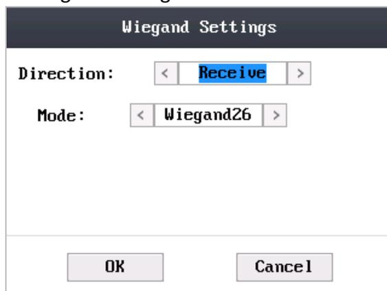
3. Edit parameters of the serial port, including the Wiegand direction and the Wiegand mode.
