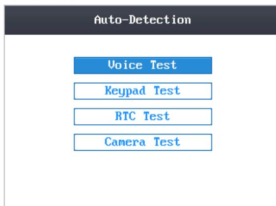
3. Move the cursor to select Voice Test, Keypad Test, RTC Test, or Camera Test to do corresponding test.
