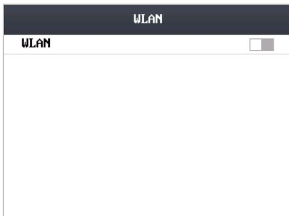
3. Move the cursor to  and tap the # key to enable the WLAN.
