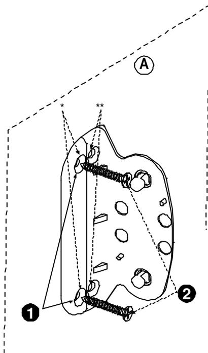
1. Drill two holes in the mounting surface.
