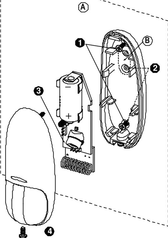
1. Drill two holes in the mounting surface and secure the base with two screws.
