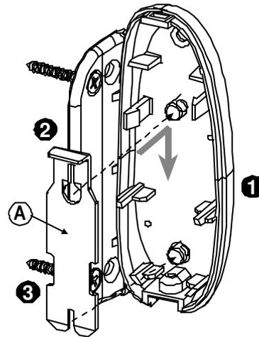
1. Place the base slots over the two bracket pins.
