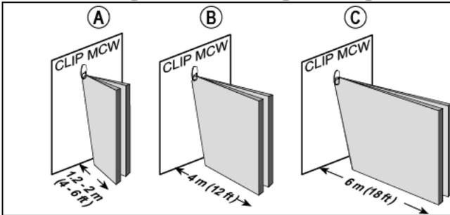
The CLIP PG2 can be programmed to select one of three ranges, according to the type of installation, for the curtain beams (see Figure 15 and section 2.7).
