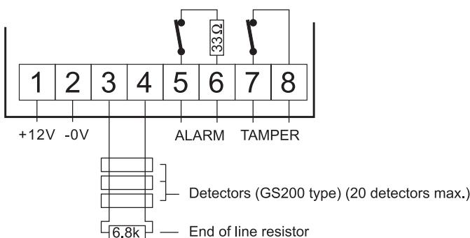
The GS218N is an interface unit that can be used when you want to connect the GS200 glass break detectors for balanced DC loops to a control panel without balanced loop connection.
