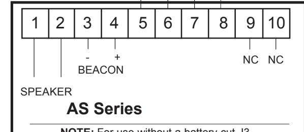
To be connected to an external current limited power supply. (Advised: 5 Amp.)
