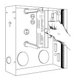
Inside the can, several 2-holed insertion points have been constructed. This allows for either vertical or horizontal placement of the modules. Notice that each insertion point has two sizes of holes – a larger hole and a smaller hole.
