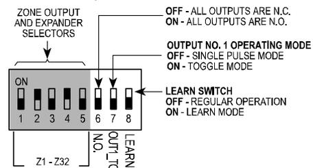
Figure 7. DIP Switch Tasks and Positions
