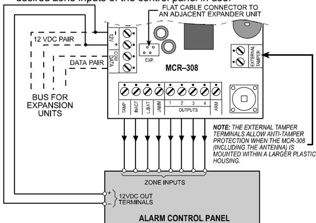
Figure 5. Wiring Diagram
