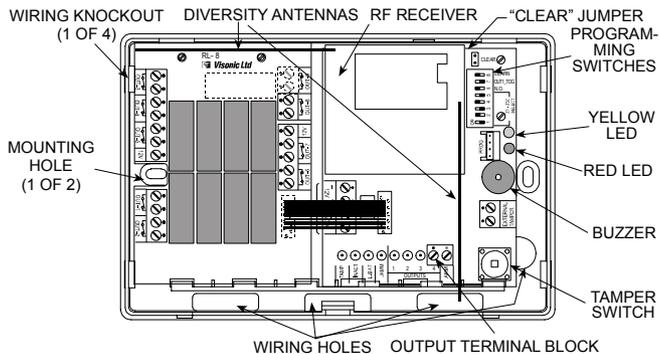
Figure 3C. MCR-308TRL with Cover Removed
